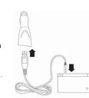
2 Insert the DC car adapter into a standard 12V DC car cigarette lighter or accessory socket. Make sure that the plug is fully inserted into the socket. The charge indicator LED on your console turns orange while recharging,
